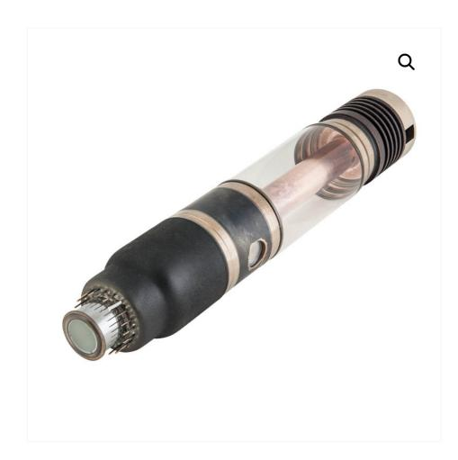
X-ray tube with cold cathode (PRT) uses built-in photomultiplier tube (PMT), as a source of electrons, instead of traditional cathodes. X-rays are adjusted by light hit the PMT photocathode. Light-emitting diode, lamp or any other source can be used as the light source. PRT can be applied in medicine (X-ray tomography), biology, x-ray space communications, in equipment for X-ray structure and X-ray spectral analyses.
