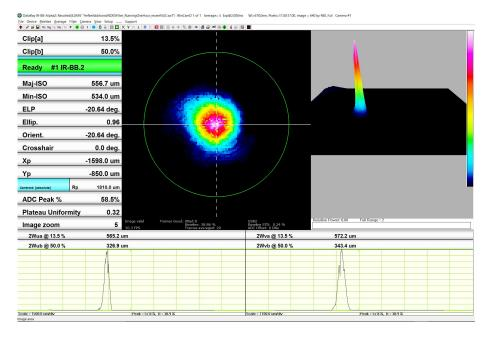
The WinCamD-IR-BB is supported by DataRay's full-featured, highly customizable, user-centric software which has no license fees, unlimited installations, and free software updates. The software supports M<sup>2</sup> measurements using our M2DU stages.
