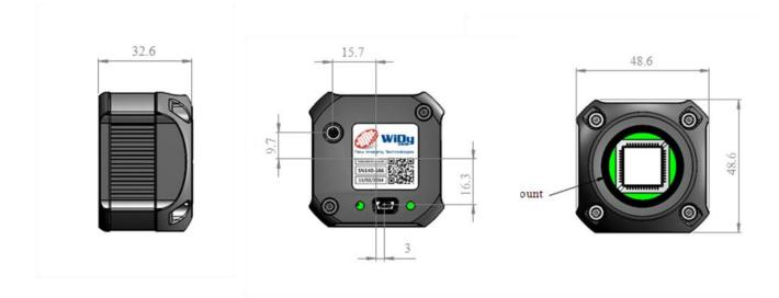
Figure 7 - WiDy 640U-S Dimensions (mm)
