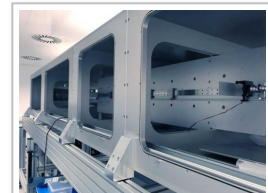
VOLCANO 750UV-6 Laser Optics for 6x TruMicro 8320 UV Solidstate Laser
