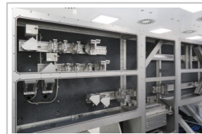
VOLCANO 300UV laser optics with two TruMicro 8320 or a single TruMicro 8340.
