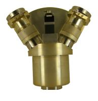
The Resonance Ltd. vacuum monochromator and spectrometer uses standard connections to allow simple integration into most systems. The f/4.2 grating is a type 4 for minimal aberrations. It is designed to allow easy interchangeability between being a monochromator with servo-controlled drive and a CCD-based spectrometer. It's supplied with LabView-based codes and drivers for integration into user software.
