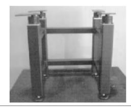
Our sturdy support stands are constructed of 3" square steel tube legs and 2" square steel cross bars. The standard support stand has leveling feet that are height adjustable +/- 1 - 2 inches. Locking casters or leveling casters are optional.
