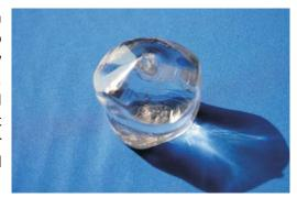
BBO has electro-optic coefficients g11=2.7pm/v, g22, g31<0.1g11. It can be used for Q-Switching a cw diode pumped Nd:YAG laser with average power>50W.
