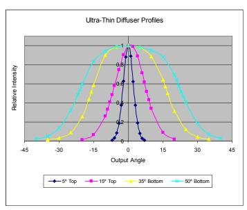
The grpah above represents data gathered from a collimated point source normal to the TMD.
