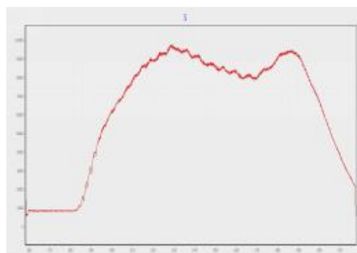
185-320nm Deuterium lamp spectrum
