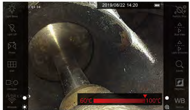
100°C resistance warning & auto shut down protection.
