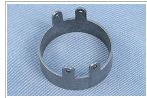
Conventional machining = multiple processes Laser tube cutting = only 1 cycle
