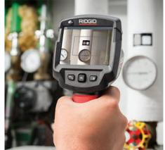
ε-Assist allows you to automatically set emissivity and reflected temperature utilizing an integrated digital camera.
