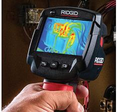
SuperResolution effectively doubles the resolution of your camera, allowing greater detail to detect anomalies.
