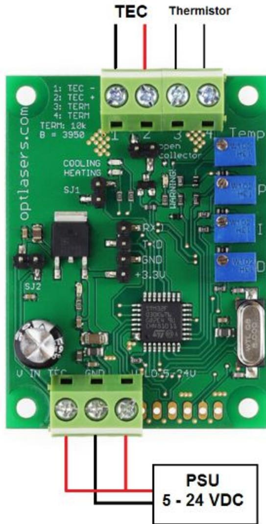
3. Using one PSU with **closed SJ2**:
