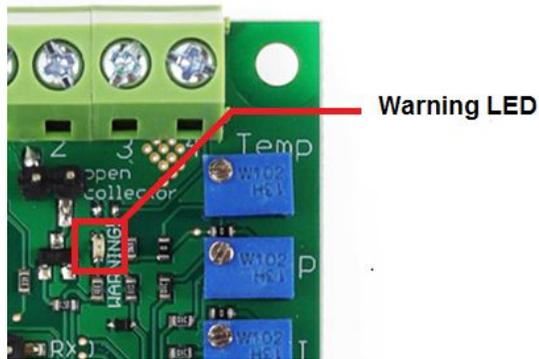
5. If the measured temperature lies between  $+45^{\circ}\text{C}$  and  $T_{\text{max}}$ , the WARNING LED is flashing. The open collector output (OC) is not connected to ground. The PID regulator works normally (unless the overriding limit mentioned before is exceeded).
