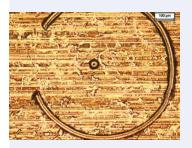
Chromium PVD layer on steel, possible corrosion site, 50 x
