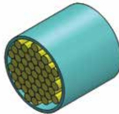
Duct containing 48 x Ø 3mm cable
