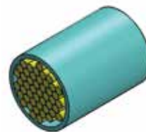
Duct containing 48 x Ø 2mm cable
