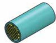
Duct containing 48 x Ø 1.2mm cable
