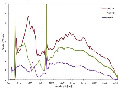
Violet (EXU), Blue (EXB), White (EXW) and Red (EXR) systems provide users with a comprehensive coverage of the supercontinuum spectrum in the 400-2400 nm range.
