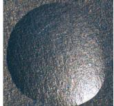
CHI-BLUE coated Be exposed to a 1 M HCl solution shows no corrosion holes after several hours.
