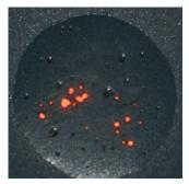
Uncoated Be exposed to a 1 M HCl solution shows many corrosion holes (orange dots) within 30 minutes.
