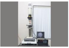
We have all the required test equipment to provide our customers with fully tested, high quality optics. We have a Fujinon F601 Spherical Surface Tester that allows us to measure the form irregularity of spherical surfaces and also measure the Radius of Curvature. We also have a Spectrophotometer for coating transmission measurements. We have a focometer with rotation stage for measuring BFD and Centration error. For more details, go to our Test Facilities.
