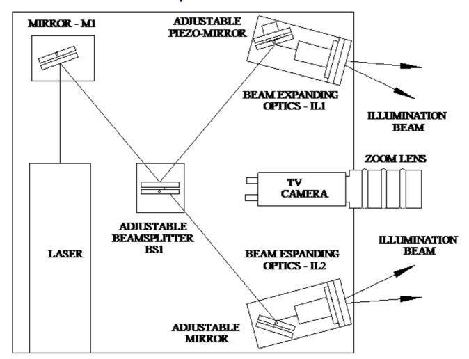
This diagram illustrates the modular design of the Electronic Speckle Correlation optical head mounted on an 18-inch square pallet. It is composed of 5 small modules, which manipulate the laser beam and divide it into two illumination beams that illuminate the object from two equal and opposite angles.
