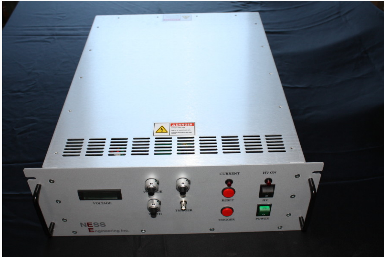
2 kV Magnetic Core Tester Top View
