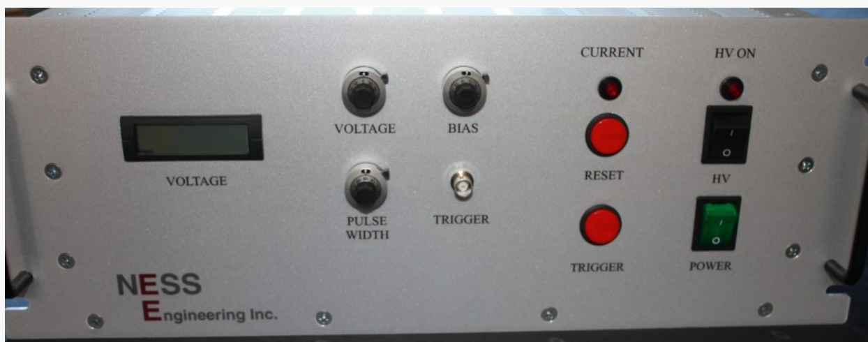
2 kV Magnetic Core Tester Front View
