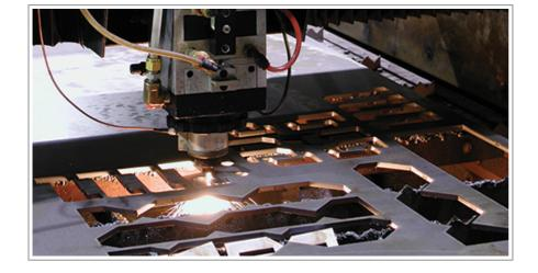
Our CO2 and fiber laser cutting systems offer rapid cutting speeds, excellent cut edge quality, minimal tapered kerf, and tight tolerances (held to  $\pm$  .005" depending on material and thickness), enabling them to perform tasks that would be difficult using conventional machinery.
