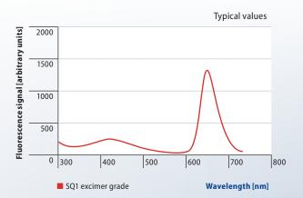
Red fluorescence: sensitive criterion for NBOHC (Non Bridging Oxygen Hole Center). Very low level is characteristic for a high Hydrogen content.
