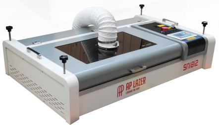
This portable small laser engraving machine allows for on-the-spot engraving. With a 30 watt laser, it is ideal for both travelling and home use.
