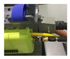
Universal mounting rails transform the handheld system to over-the shoulder or robot-mounted
