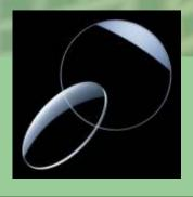
Anti reflection coatings are transmission enhancement coatings which when deposited on the optics will increase the through put into the optical system, reduce the stray light, and prevent the back surface multiple reflections. They are broadly divided in to three types. Single layer, V-type, broadband coatings.
