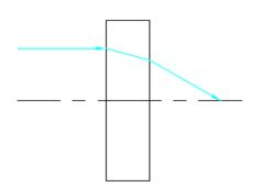
Rod Cylindrical Lens are used to focuses Collimated Light into a Line who act as a Bi-Convex Cylindrical lenses.
