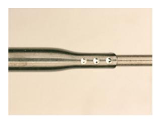
The image pictured above is one example of this type of assembly. Two different hypotubes go through multiple processes at Resonetics before being joined together via laser welding. The larger hypotube on the left is laser cut and formed to fit the smaller hypotube, then tumbled to break the edges. The smaller hypo tube on the right is EDM cut to length. This example is often used for neurovascular and peripheral vascular devices.
