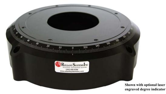
The RSR is a low profile, high precision rotary stage driven directly by an integrated brushless motor in place of a mechanical worm gear or belt drive. Benefits include no backlash, better positioning sensitivity, higher speeds, smaller envelope, and no drive wear and maintenance. This makes the RSR's well suited for applications that require high rotational accuracy, excellent positioning sensitivity and repeatability, and fast move and settle times.
