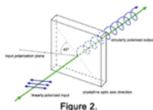
When linearly polarized light is input at 45deg to the axis of a quarter waveplate , the output is circularly polarized similarly, input circularly polarized light is transformed into linearly polarized light.
