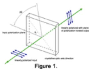
A half waveplate rotates linearly polarized light to any desired orientation. The rotation angle is twice the angle between the incident polarized light and optical axis.
