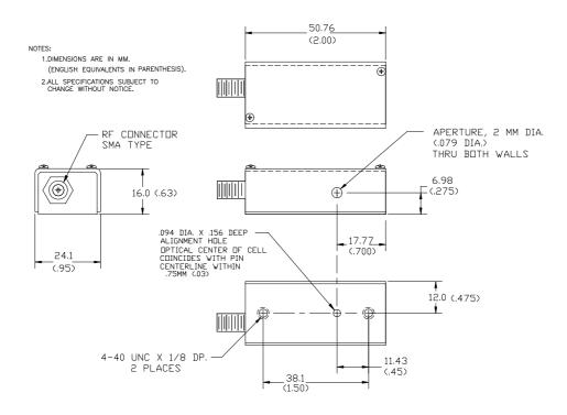
Ensure adequate heaksinking through mounting surface, especially at higher RF powers.
