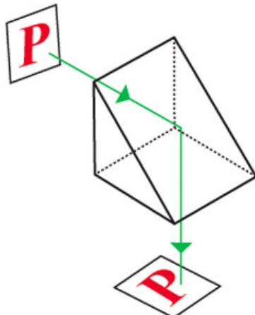
Commonly used to create a 90° bend in the light path, these prisms present images two ways depending on their orientation. In the first, images will be inverted but positioned correctly left to right. Rotate the prism 90°, and images will be right side up, but transposed horizontally. Several right angle prisms can be combined to achieve image/beam displacement. Angular tolerance  $\pm 2$  arc seconds, surface quality 20/10, surface accuracy  $\lambda/10$ , dimensional tolerances  $\pm .002"$ .
