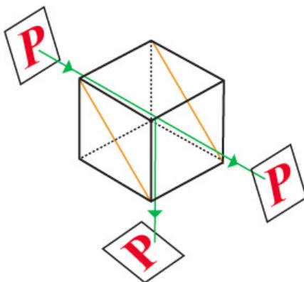
These optical components are made by cementing two precision right angle prisms together and covering their hypotenuse surface with an interference coating. (Absorption loss caused by the coating is minimal.) On average, nearly 50% transmission and reflection can be produced, although it is partially polarized. In general, material is BK7, angle tolerances to < 1 arc second, flatness to  $\lambda/10$ , surface quality 20/10, dimensional tolerances  $\pm .002"$ .
