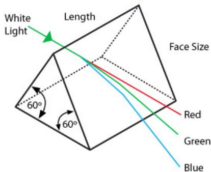
Also called dispersing prisms, equilateral prisms have three equal  $60^\circ$  angles. Angular tolerance  $\pm 5$  arc minutes, surface quality 60/40, surface accuracy  $\lambda/10$ , dimensional tolerances  $\pm .002"$ .
