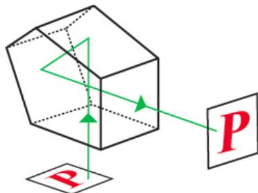
These five-sided prisms deviate beams by 90 degrees, independent of the prism's orientation - without inverting or reversing the image. Due to geometry, the reflecting surfaces must be aluminized. Penta prisms are often used to shorten the length of an instrument's optical path. All dimensions are in mm. Angular tolerance  $\pm 2$  arc seconds, surface quality 20/10, surface accuracy  $\lambda/8$ , dimensional tolerances  $\pm .002"$ .
