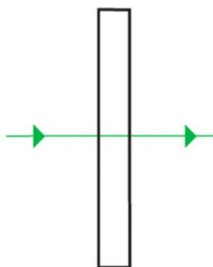
PG&O windows are optimally suited to applications demanding minimal deviation in the transmitted beam. Commonly offered in BK7 or Fused Silica, they may be ordered in a range of other optical materials as well. We can achieve a parallelism specification of  $< 1$  arc second and flatness to  $\lambda/20$ . Tolerances are typically held to  $\pm .001"$  and surface quality to 10/5.
