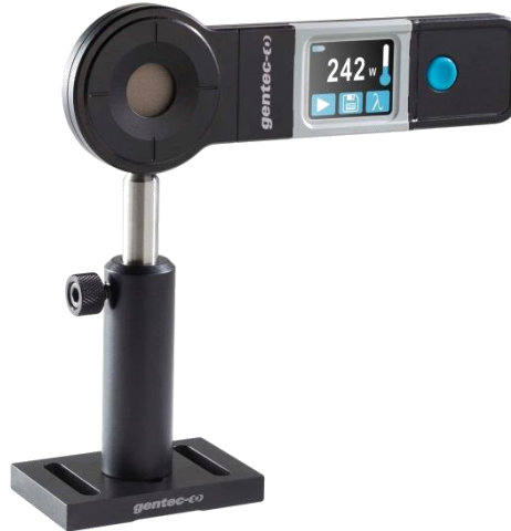
Figure 8 Recommended setup when making a measurement: install the device on an optical stand before placing it in the laser beam path.
