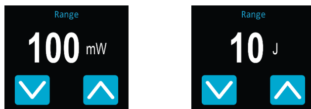
Figure 7 In the Range menu, use the Up and Down buttons to set the manual range or to go back to the default “Auto” range setting.
