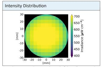
Typical 280nm Irradiance at the end of the collimating tube. Data taken from a PearlLab Beam S280 using SED270/Q5 detector.
