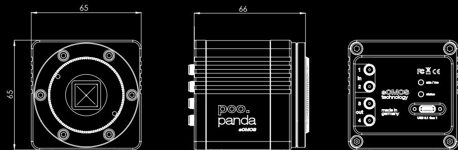
F-mount and C-mount lens adapter are changeable. All dimensions are given in millimeter.
