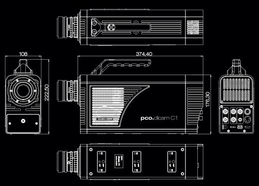
All dimensions are given in millimeter.
