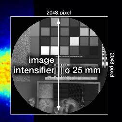
The projected image circle is completely covered by 2048 x 2048 6.5 µm pixels of the sCMOS detector – cf. image left. There is no "waste" of valuable intensifier area. As a consequence the four corners of the sCMOS sensor remain black. For a fast scan of just a few vertically centered lines – the camera module allows for more than 1.000 fps for such a ROI - the full line length of 2048 pixels is available.
