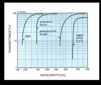
Typical transmittance of image intensifier input window materials
