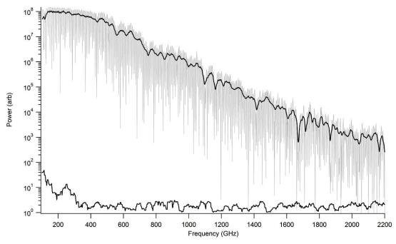
Air at 1 ATM with water vapor. No processing was performed because head spacing was adjusted to remove interference fringes from the region of interest.
