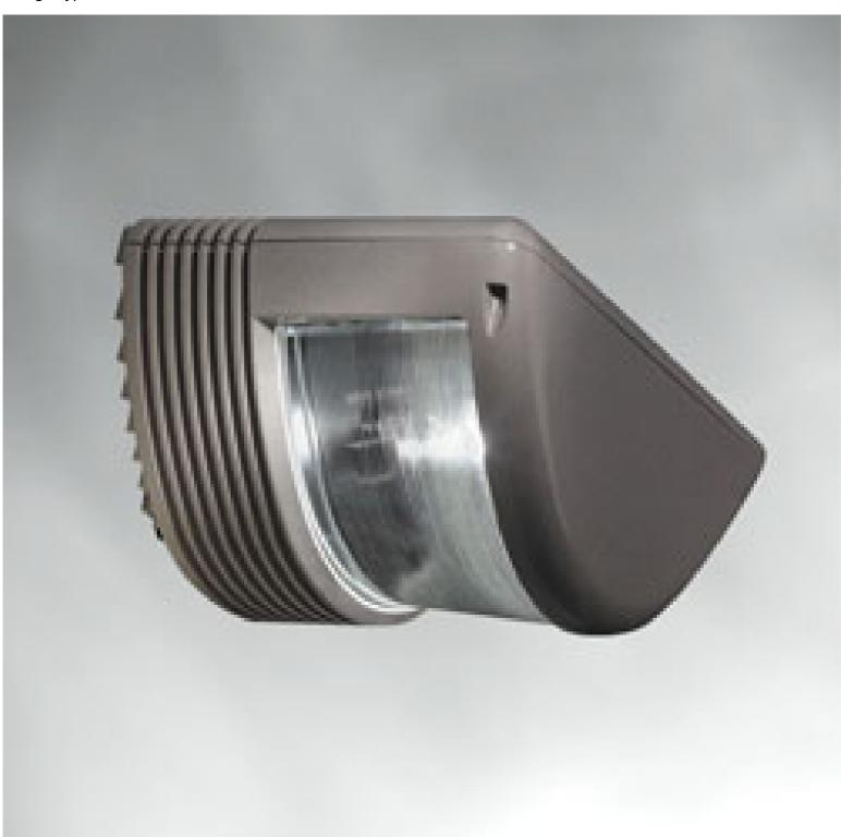
The Fascia Wash is a wall mounted luminaire designed to light large wall surfaces as evenly as possible with as wide a spacing as possible. The luminaire offers an alternative to floodlighting which requires luminaires mounted away from the building. A barrel style Fresnel lens was used in conjunction with internal reflector optics to produce the desired performance. The luminaire stands only 14" off of the wall surface yet achieves a mounting height of 20' and a spacing of 40'.
