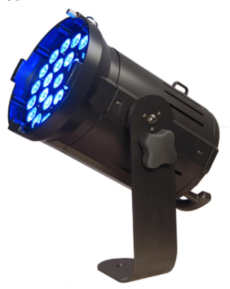
Narrow beam RGBW color changing theatrical light. Each TIR lens has an LED with RGBW in a single TIR lens to minimize rainbow edges in shadows. Optics mix all colors smoothly over the beam, while maintaining tight beam control.
