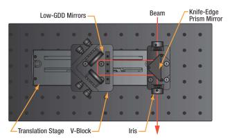
The precise positioning and stability of the low-dispersion mirrors on the direct drive stage enables sub-femtosecond delay resolution.
