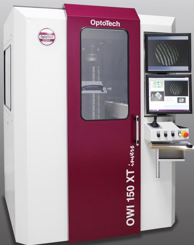
High precision Fizeau workshop interferometer OWI 150 XT invers for testing of spherical and aspherical surfaces. High precision kinematics and a working range up to  $\varnothing$  150 mm make this measuring machine an indispensable tool for the production of high-end optics.
