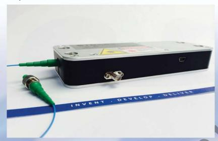
The 1 Micron Narrow Linewidth Laser Module houses a proprietary driver/controller and the OEwaves laser source which is based on a high quality factor (Q) Whispering Gallery Mode (WGM) micro-resonator. The laser is scalable to a variety of wavelengths within 980-1080 nm range.
