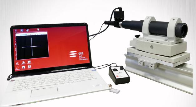
Autocollimator with infrared camera and live image transmission of the measurement to the computer
