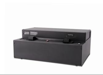
The AUTOSTRIPPER $^{\text{TM}}$  is designed for fast, chemical free window stripping of optical fibers, using heated air to accomplish the often difficult task of window stripping fibers with acrylate coating diameters up to 550  $\mu m$ .
