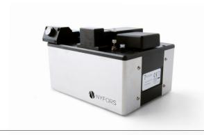
The AUTOCLEAVER S2™ is an automatic system for precision cleaving of sensitive air-clad and microstructured fiber. It has a specially designed clamping system with air pressure controlled force regulation that enables it to clamp and hold also brittle specialty fibers that might otherwise be damaged during cleaving.
