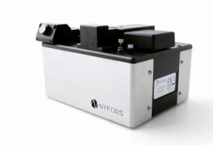
This fully automated optical fiber cleaver is designed for fast and flexible large diameter fiber processing in factory and laboratory environments. Easily interchangeable fiber handling parts enable high precision cleaving of different circular fibers in the range from 230  $\mu$ m up to 1000  $\mu$ m cladding diameter with industry leading repeatability and consistency.
