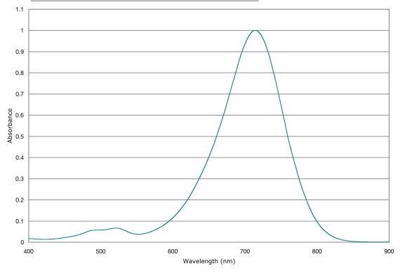
NIR714A is one of many Near Infrared (NIR) Dyes for solvent systems available through QCR Solutions Corp. We offer NIR dyes in a wide spectral range between 714nm -2000nm for various applications. Our large library of absorbers contains narrow notch to broad band absorption curves. These NIR dyes can be used singly or in combination to create custom spectral filters.
