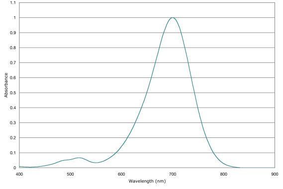
**NIR700A** is one of many Near Infrared (NIR) Dyes for solvent systems available through QCR Solutions Corp. We offer NIR dyes in a wide spectral range between 700nm -2000nm for various applications. Our large library of absorbers contains narrow notch to broad band absorption curves. These NIR dyes can be used singly or in combination to create custom spectral filters.
