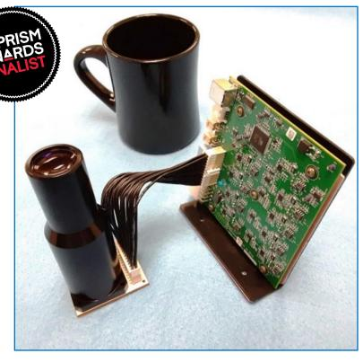
Consuming only 15W of input power, it is energy efficient and simplifies any thermal interface or active cooling scheme. The compact and lightweight design supports a diversity of system integration concepts previously unattainable. The extensive value proposition offers lower power, higher stability, smaller size, greater application flexibility, and a significantly lower cost-of-ownership for PV testing compared to other commercial solar simulators.
