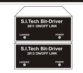
The S.I.Tech Model 2811 TR transmits a 10 KHz optical square wave over optic fiber when power is applied and control input shorted. The 2812 receiver detects this optical square wave and turns ON a 4PDT relay. If the fiber cable is removed, broken, or the remote transmitter or local receiver loses power, the relay in the local receiver will turn OFF.
