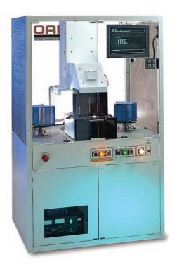
OAI MODEL 2000 **EDGE-BEAD AND UV FLOOD EXPOSURE SYSTEM**
